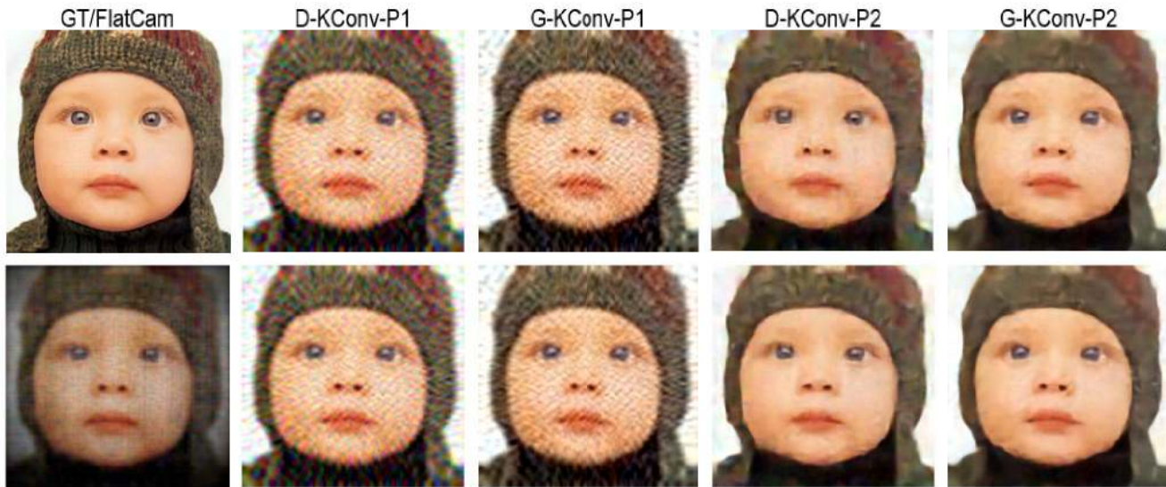
Figure 6. Quality of visual reconstruction for simulated Baby FlatCam data. First row - ground truth and reconstructed images from standard network. Second row - conventional FlatCam [25] and reconstructed images from residual network
