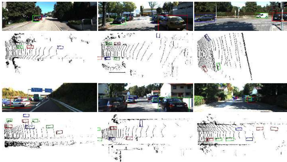
Fig. 4: Qualitative results on KITTI Dataset. The BEV-image pairs and the detected bounding boxes are shown. The 2D bounding boxes are obtained by projecting the 3D detections onto the image. The bounding box of an object on BEV and images are shown in the same color.
