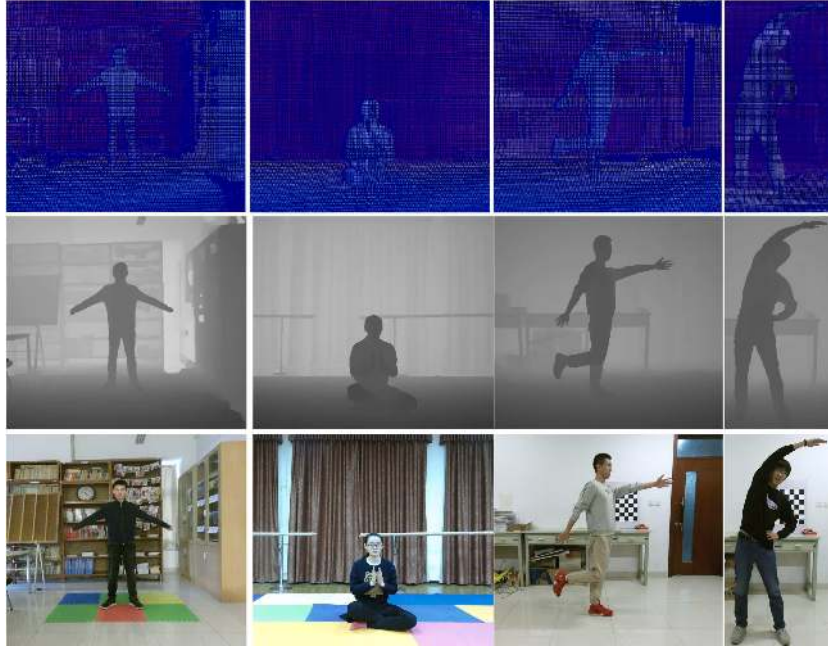
Figure 9: Some examples in our constructed real-world RGB-D dataset. The first row represents the warped degraded depth images, which are captured by Kinect-v2 and then warped based on camera parameters. The warped degraded depth images have the same view and size as the corresponding color images shown in the third row, and meanwhile have structure missing and random missing. The second row represents the pseudo GT. The third row represents the high-quality color image captured by Kinect-v2. To better visualize degraded LR depth maps, we show the colorized version.
