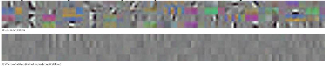
Figure 7. Visualization of Conv1a filters learned by C3D (top) and V2V (bottom). Note that C3D is trained to recognize actions (on Sport1M), while V2V is optimized to estimate optical flow (on UCF101). Each set shows the 64 learned filters at the Conv1a layer. Three consecutive square images on each row represent one filter (as kernel size is 3 \times 3 \times 3 ). Each square image is upscaled to 30 \times 30 pixels for better visualization. Best viewed in color. GIF animation of these filters will be provided in the project website.
