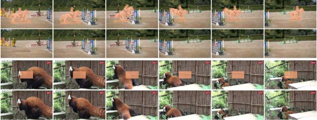
Figure 6: Results of our flow-guided video inpainting approach. For each input sequence (odd row), we show representative frames with mask of missing region overlay. We show the inpainting results in even rows. Best viewed with zoom-in.
