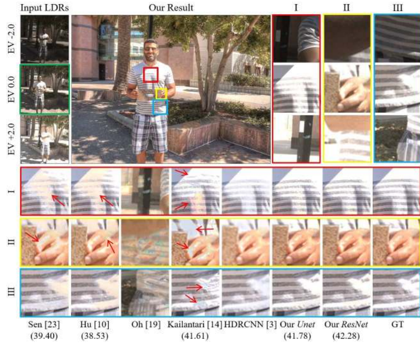
Fig. 3. Comparison against several state-of-the-art methods. In the upper half of the figure, the left column shows in the input LDRs, the middle is our tonemapped HDR result, and the last three columns show three zoomed-in LDR regions marked in the HDR image. The lower half compares the zoomed-in HDR regions of our results against others. The numbers in brackets at the bottom indicate the PSNR of the tonemapped images. Images are obtained from the Kalantari’s test set [14].
