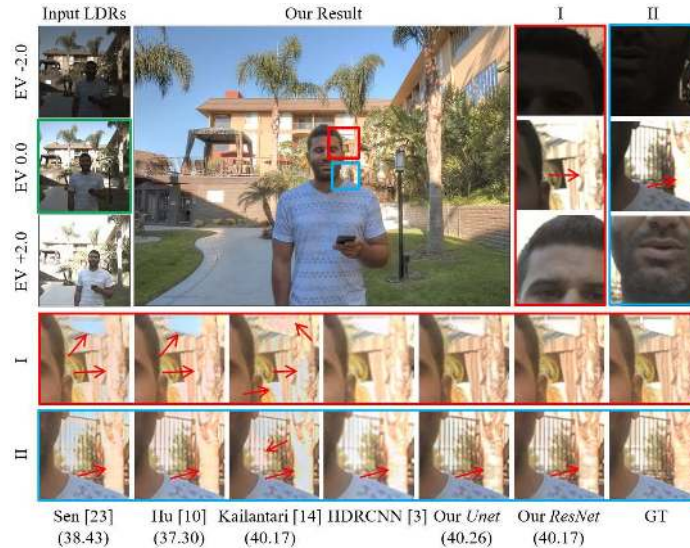
Fig. 6. Comparison of hallucinated details. Our network hallucinates the missing trunk texture, while others may fail. Images are obtained from the Kalantari’s dataset [14].
