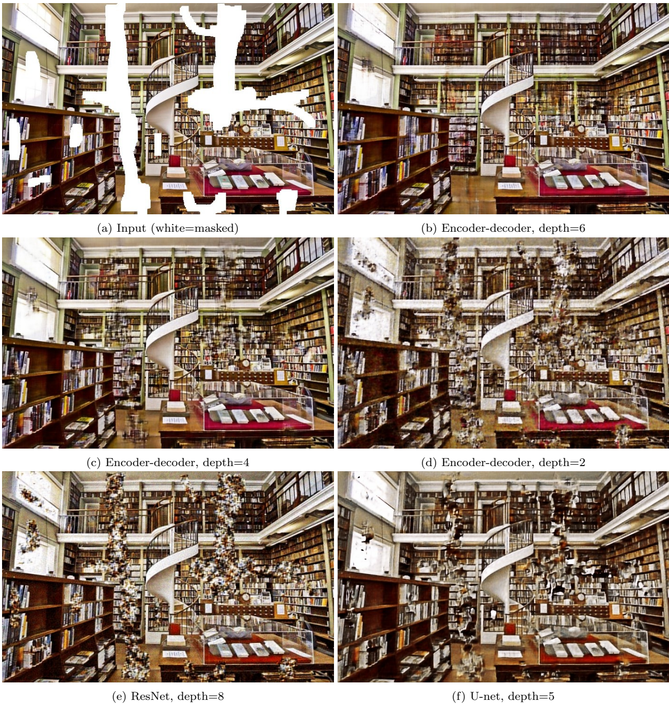
Fig. 14: Inpainting using different depths and architectures. The figure shows that much better inpainting results can be obtained by using deeper random networks. However, adding skip connections to ResNet in U-Net is highly detrimental for the deep image prior.
