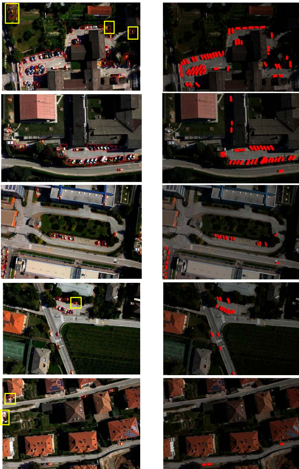
Figure 10. Detection results of the proposed algorithm for Test Images 1–5 together with their ground truths. Particularly difficult cars that were detected by the proposed algorithm are highlighted with yellow boxes.
