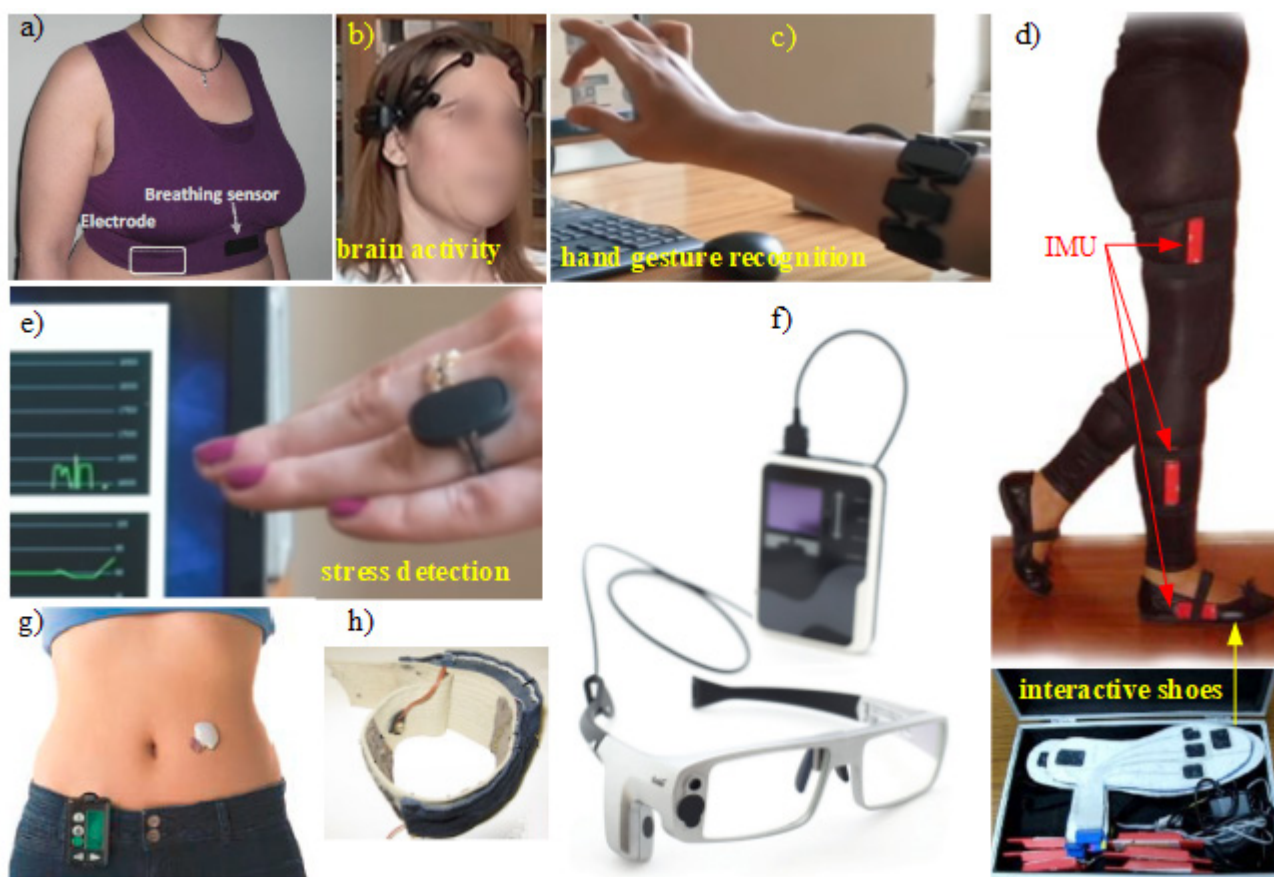
Figure 2. a) Wearable Wellness System from (8), b) Emotiv EPOC ® neuroheadset, c) Myo armband ® hand gesture controller, d) SENSY system for gait analysis (17), e) Moodmetric ® ring for stress follow, f) Tobii ® eye tracker glasses form (20), g) Medtronic ® continuous glucose monitor form (21), h) A prototype of wearable 24-hour blood pressure device form (22)
