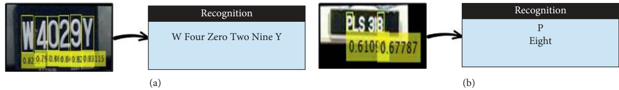
FIGURE 12: Malaysian result of (a) correct and (b) wrong recognition (YOLOV2).
