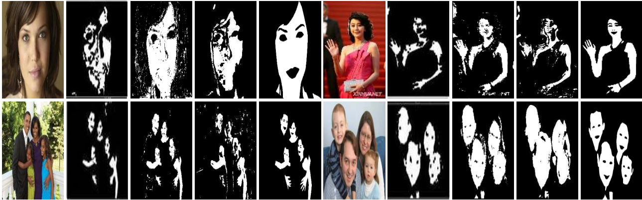
Figure 4. Comparison with [31]: The first and sixth columns show original images. Second and seventh columns show the output of [31]. Third and eighth columns show skin segmentation obtained by our patch-based CNN (Fig. 3 (a)). Fourth and ninth columns show skin segmentation obtained by our regression based CNN (Fig. 3 (b)). Fifth and tenth columns show ground truth images.
