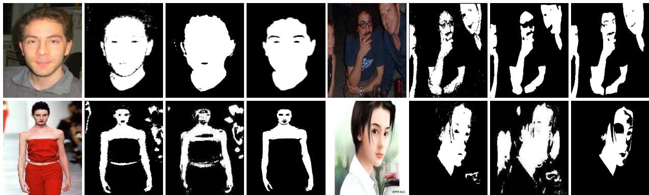
Figure 5. First row shows the skin detection result on Uchile dataset [43] and second row shows the result on IBTD dataset [44]. First and fifth columns show original images. Second and sixth columns show segmentation results of our patch-based skin detection algorithm (Fig. 3 (a)). Third and seventh columns show segmentation results of our regression based skin detection algorithm (Fig. 3 (b)). Fourth and eighth columns show ground truth images.
