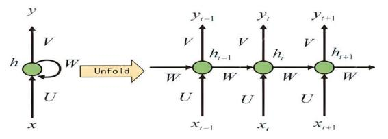
Figure 4. An illustration of the RNN model.
