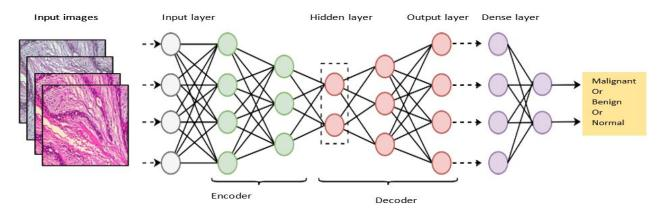
Figure 2. An illustration of the deep autoencoder.
