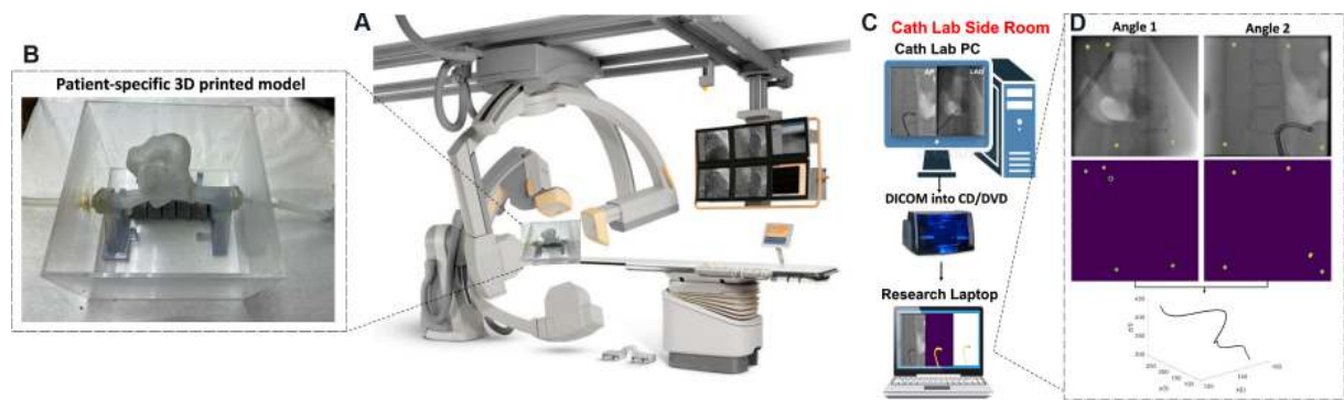
Figure 1. Schematic of the proposed training system. (A) Image of 3D printed heart model on a bi-plane c-arm. (B) Magnified view of patient-specific 3D printed heart model. (C) Schematic of image transfer process and post-processed catheter tracking. (D) Image-processing and deep learning steps of bi-plane images with tracking plot.
