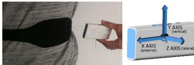
Figure 3: The data collector IMU and its location on patients’ body (i.e. left side of their waist).
