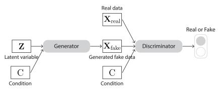
Figure 17. Diagram of a cGAN.
