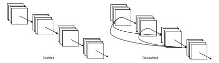
Figure 6. DenseNet block vs. ResNet block.
