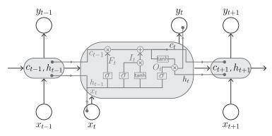
**Figure 11.** Diagram of a LSTM memory cell. c, h are the cell state and hidden state, respectively, t is the time, and  $F_t$ ,  $I_t$ ,  $O_t$  are the forget gate, input gate, and output gate, respectively.
