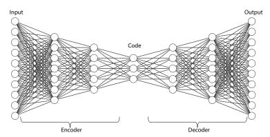
Figure 13. Diagram of an AE.
