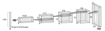
Figure 16. Diagram of a DCGAN.
