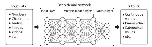
**Figure 1.** Diagram of a DNN.
