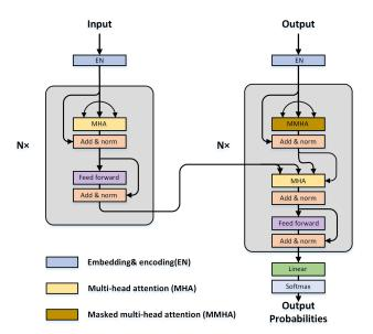
Figure 18. The model architecture of the Transformer.
