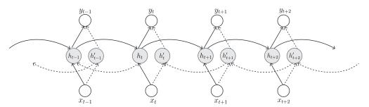
**Figure 10.** Diagram of a BRNN. x, y represent the input and output, respectively, h, h' represent the two bidirectional memory units, and t is the time. Solid arrows represent data forward propagation, and dashed arrows represent data back propagation.
