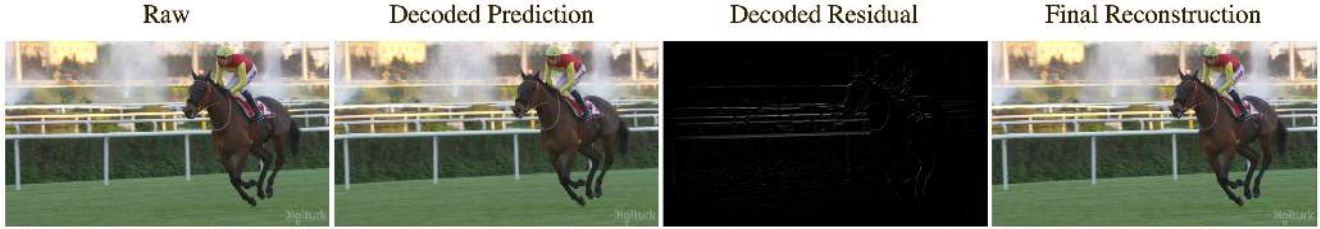
Figure 5. Visualization of our model results. The prediction network predicts for the next-frame latent according from several preceding latents (second left). The residual (second right) in the latent space is added to the predicted latent for final reconstruction via the generator.
