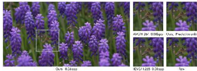
Figure 1. Reconstructed frame with the conventional codecs (H.264, H.265) and our approach. Information and details are well preserved in the frame generated from a purely prediction-based latent representation (top right). Compared with H.264, our result yields less block artifacts and preserves finer details. Our method achieves a higher compression ratio than H.265 with similar quality.
