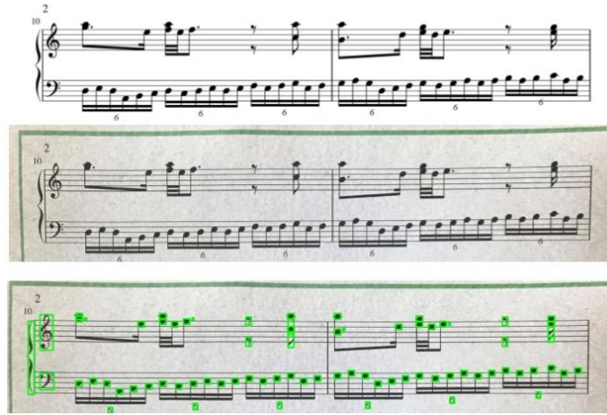
Fig. 10: Top: part of a synthesized image from DeepScores ; middle: the same part, printed on old paper and photographed using a cell phone; bottom: the same image, automatically retrofitted (based on the dark green lines) to the original image coordinates for ground truth matching (ground truth overlaid in neon green boxes).
