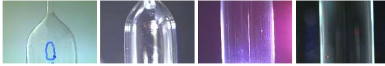
Fig. 5: Balloon catheter images taken under different optical conditions, exposing (left to right) high reflections, low defect visibility, strong artifacts, and a good setup.
