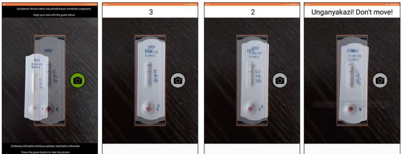
Extended Data Fig. 2 | Screenshots of the Android application, to illustrate the capture of the HIV RDT image at the time of reading the test result. Images were captured sequentially from left to right. The end user is asked to align the test with the overlay on the screen, then continuously press the capture button for 3 seconds, after which the image is automatically captured and processed to extract the ROI. The 3 seconds press feature was implemented as a result of consultation with end users in the optimisation phase of the app development.
