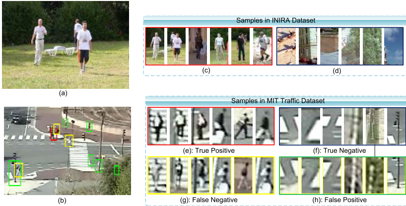
Fig. 1. (a): Image from INRIA dataset. (b): Image from MIT Traffic dataset. (c): Positive samples in INRIA. (d): Negatives in INRIA. (e)-(h): Detection results of a generic detector (HOG-SVM [5] trained on INRIA) on MIT Traffic. (e): True positives. (f): True negatives. (g): False negatives. (h): False positives. Best viewed in color.
