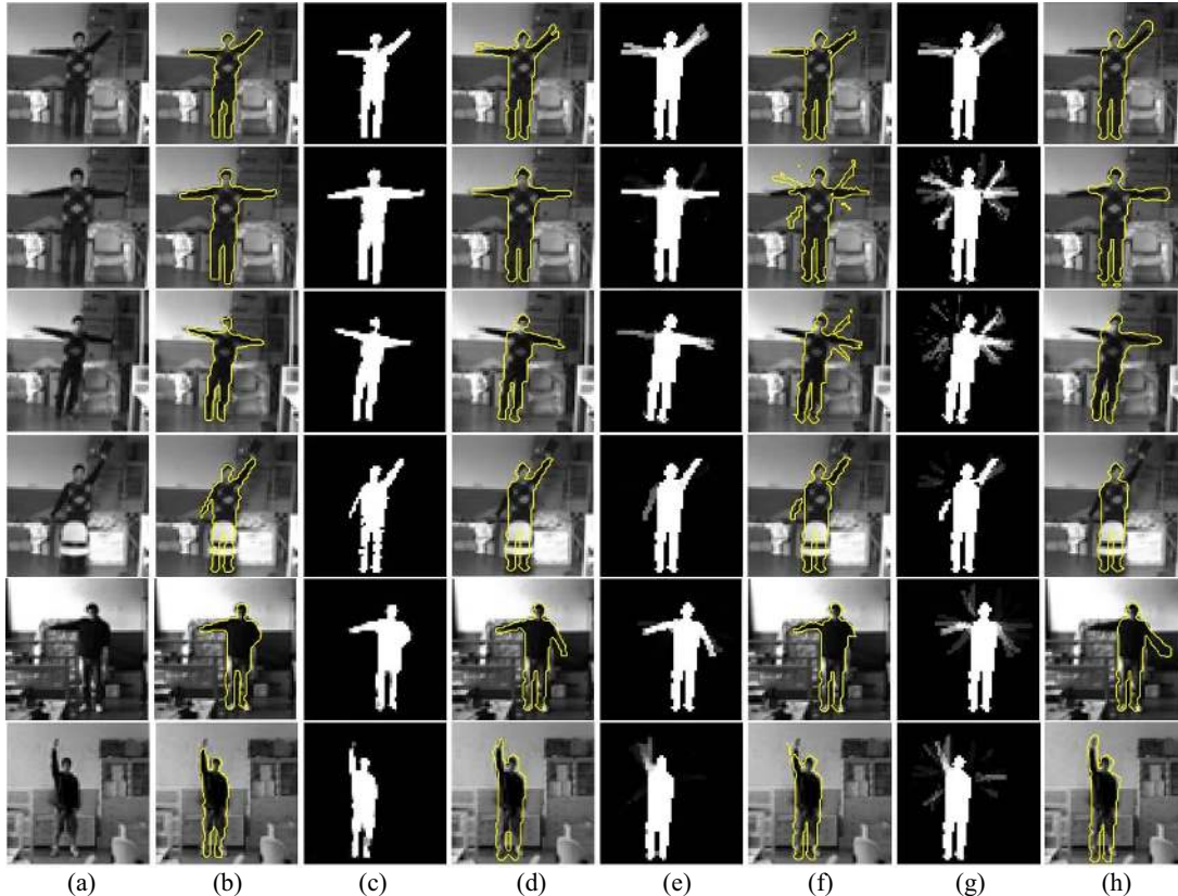
Fig. 9. Typical segmentation comparisons of four different methods. (a) Original images. (b) Results by our model, and the corresponding shapes in (c). (d) Results by shape sparse representation [11], and the corresponding shapes in (e). (f) Results by kernel density estimate of shape prior based on shape probabilistic definition [8], and the corresponding shapes in (g). (h) Segmentation results by [6].
