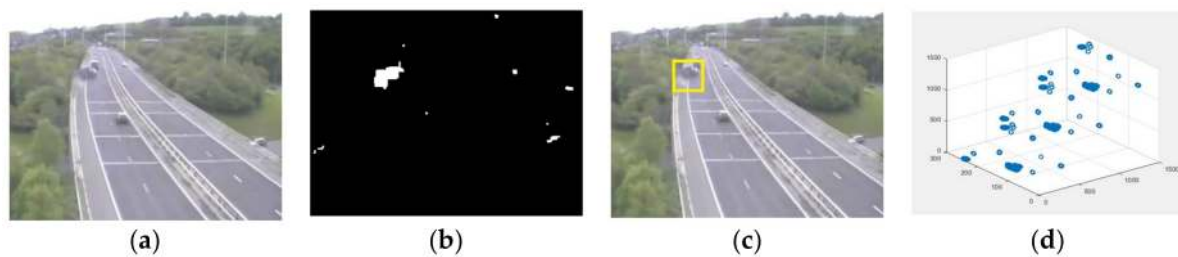
Figure 5. Illustration outlines for the LV datasets. Inconsistent occasions are featured by boxes. (a) Original image; (b) background subtraction frame; (c) abnormal event detected frame; and (d) 3D plot representation.
