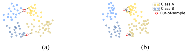
Fig. 2. Graphical illustration of the main limitation of SNCA. (a) In the metric space produced by SNCA, it will be challenging for the K NN classifier to distinguish the out-of-sample images located near the border between the two classes. (b) By introducing CE loss, these two classes are further separated in the metric space, and the same out-of-sample images in (a) can be accurately categorized by the K NN classifier.
