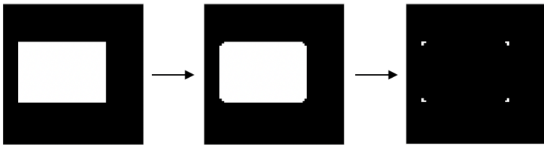
Figure 2.4 The morphological residual model. Applying opening on the original image with circle structuring elements, then subtraction of result image from original image can obtain the morphological residuals.
