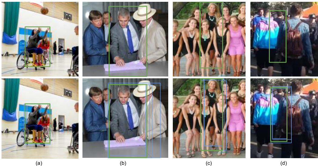
Figure 4: Mixture of Gaussians predictions. First row: baseline Faster R-CNN. Second row: mixture of four Gaussians. Blue boxes are the mixture components. Green boxes are the final predictions. (a) not occluded (b) left arm is occluded (c) both arms are occluded (d) heavily occluded.
