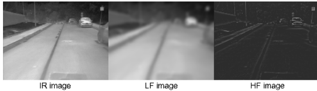
FIGURE 4. Comparison of the high-frequency (HF) and low-frequency (LF) part of infrared (IR) image. The left image is original IR image, and the middle image is LF part of IR image extracted by gaussian filters with 30 \times 30 kernel and \sigma equal to 8. The right image is the correspond HF part by the same gaussian filter.
