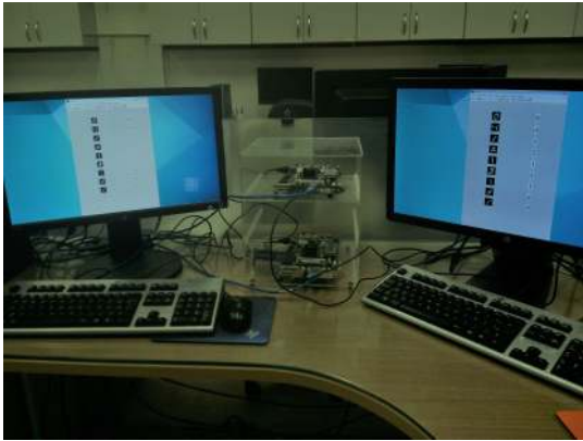
FIGURE 30. Hardware setup for the experiments with the Xilinx Virtex-6 FPGA ML605 evaluation kit.
