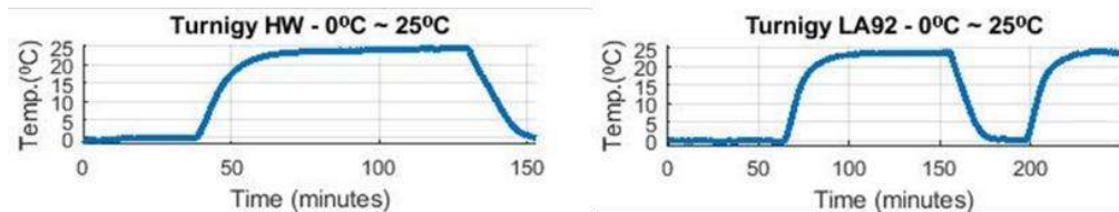
Figure 7.10 Turnigy LA92 and HW battery temperature varying from 0°C to 25°C over time.
