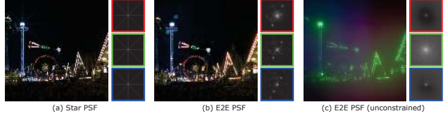
Figure 4: Simulated sensor images for an example from our evaluation set and point spread functions (PSFs) of several different optical coding approaches: (a) Rouf et al.’s star-shaped PSF [58], (b) our end-to-end optimized PSF with physically realizable constraints, and (c) our end-to-end optimized PSF without constraints. All three color channels of the PSFs are shown separately in the log domain. Whereas the star PSF continuously blurs the image along several radial streaks (a), the deep optics approach creates a PSF with several distinct peaks, which result in image content being copied at chromatically varying distances and at different intensity scales (b). The unconstrained PSF blurs the green color channel while focusing the red and blue channels.
