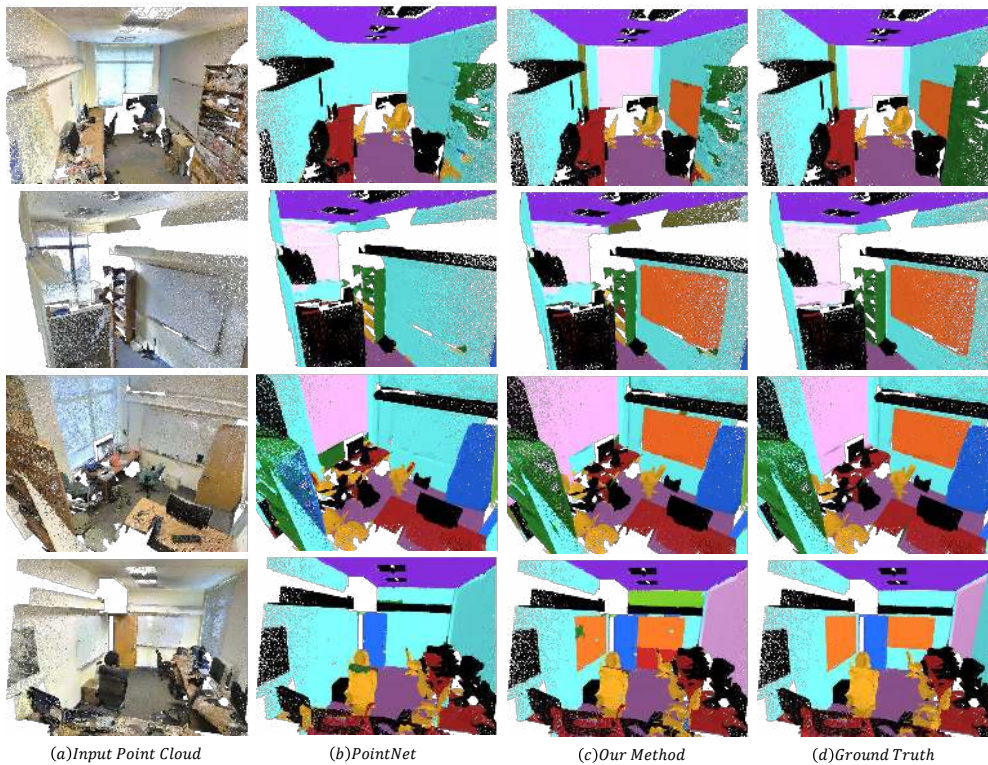
Figure 6. Comparison of results of PointNet and our method on the S3DIS dataset. For most case PointNet failed to classify the board, window and column due to its limited geometry shape feature. And our method produce less label noise as the consistent points of a single object usually share some segmentation patches in suitable segmentation level.
