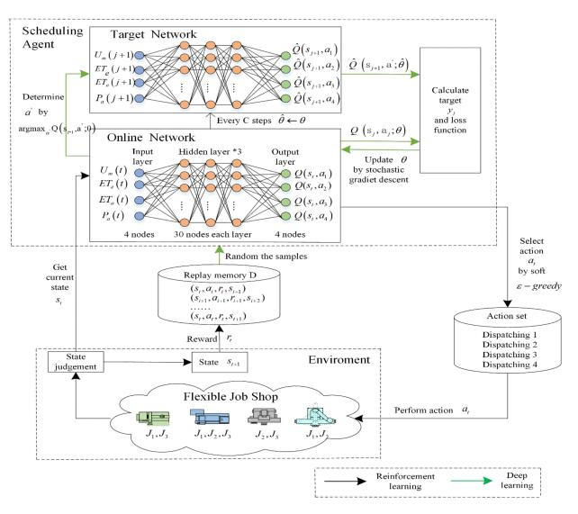
Figure 1. The model architecture of solving the DFJSP using the DDQN.
