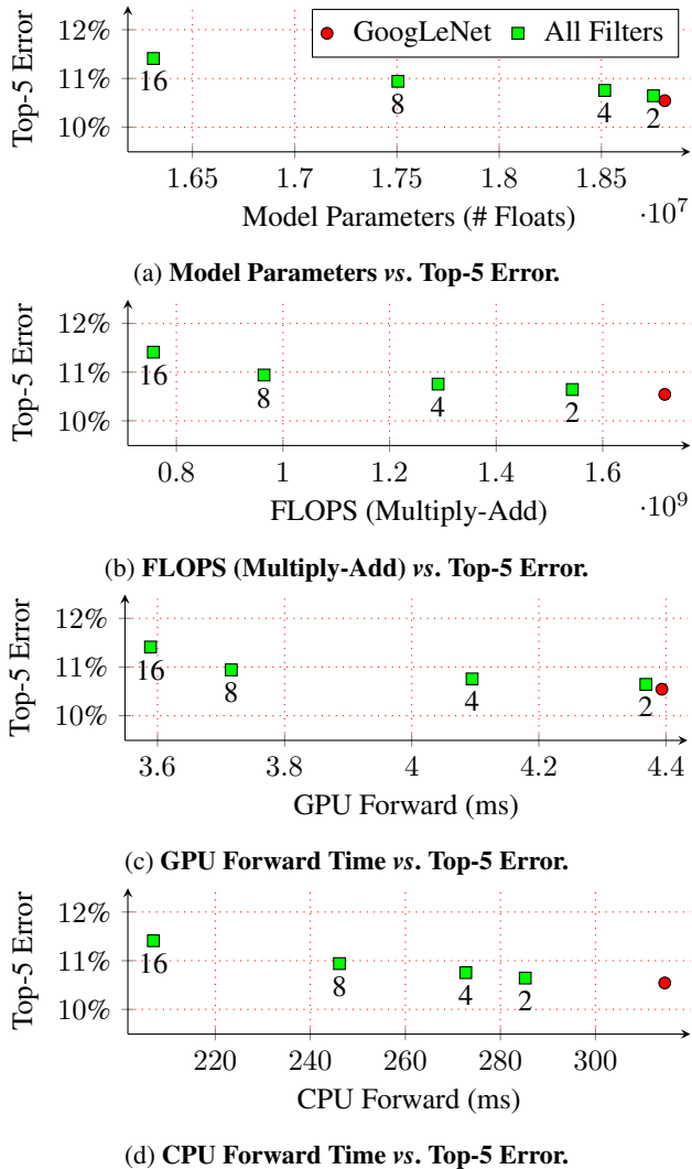
Figure 9: GoogLeNet Results. Models with filter groups have fewer parameters, and less floating point operations, while maintaining error comparable to the baseline.
