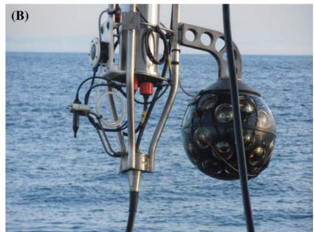
Fig. 1 a A 3D cutaway drawing of the DOM. The zenith angle \theta and the azimuthal angle \phi are indicated. Vertically upward corresponds to \theta = 0^\circ whereas \phi = 0^\circ points to the support cable. b The DOM connected to the ANTARES instrumentation line. The structure to which the DOM is connected is a standard ANTARES support frame including a cylindrical electronics container
