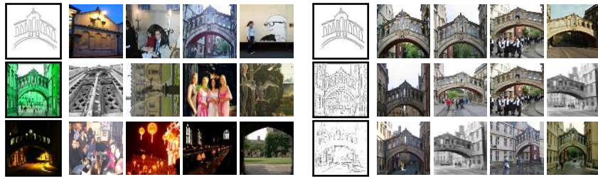
Fig. 1. Three examples where shape is the only relevant information: sketch, art-work, extreme illumination conditions. Top retrieved images from the Oxford Buildings dataset [1]: CNN with an RGB input [2] (left), and our shape matching network (right). Query images are shown with black border.
