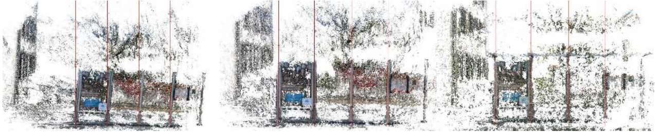
Figure 6: Generalization performance on real data. Left: Reconstructed 3D model with input rolling shutter images. Middle: Reconstructed 3D model with predicted global shutter images. Right: Reconstructed 3D model with real global shutter images.
