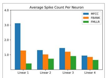
**FIGURE 5** | Average spike count per neuron of different SNN layers on the TIMIT corpus. The results of different input features are color-coded. Sparse neuronal activities can be observed in this bar chart.
