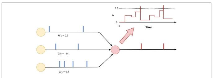
**FIGURE 3** | The neuronal dynamic of an integrate-and-fire neuron (red). In this example, three pre-synaptic neurons are sending asynchronous spike trains to this neuron. Output spikes are generated when the membrane potential *V* crosses the firing threshold (top right corner).
