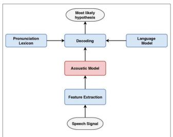
**FIGURE 2** | Block diagram of a conventional ASR system. The acoustic and linguistic components are incorporated to jointly determine the most likely hypothesis.
