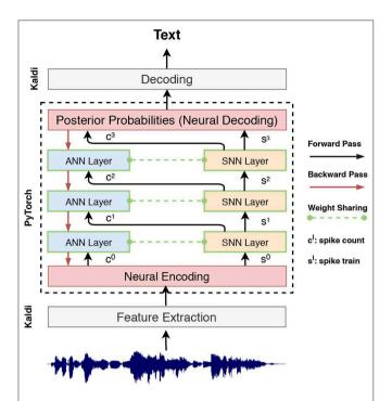
**FIGURE 4** | System flowchart for SNN training within a tandem neural network, wherein SNN layers are used in the forward pass to determine the spike count and spike train. The ANN layers are used for error back-propagation to approximate the gradient of the coupled SNN layers.
