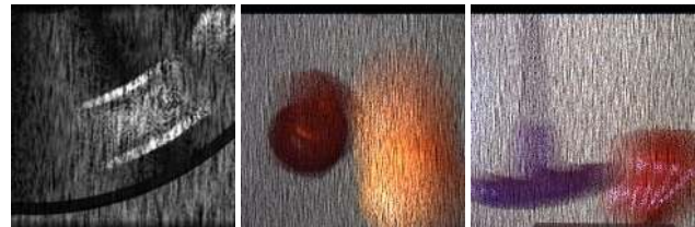
Figure 7. Real video SCI system measurements: Wheel , Balls and Hammer . Wheel : Different characters are attached on a fan while the fan is performing high-speed rotation ( B = 14 and all frames are shown in Fig. 8). Ball : Two plastic balls drop freely and hit the ground. Then, the rotation and rebounding happen on the two objects respectively ( B = 22 and every other frame is selected and shown in Fig.9). Hammer : A hammer, swinging like pendulum, knock down a plastic apple ( B = 22 and every other frame in shown in Fig. 10).
