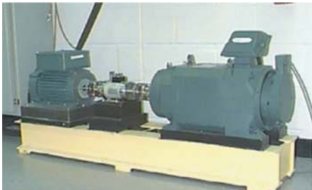
FIGURE 4: Bearing testbed used for experiment.
