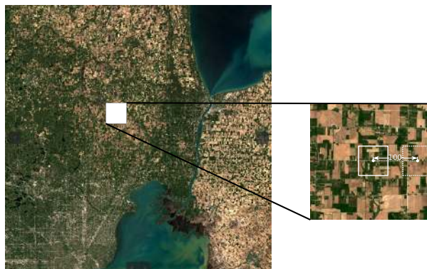
Fig. 3. Creation of a training dataset from the downloaded tile. As an example, we randomly crop one image from a Sentinel-2 tile with size of 264 \times 264 pixels, since the distance between the centers of the anchor patch and the spatially augmented patch is 100 pixels.
