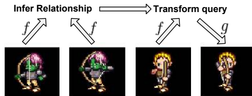
Figure 1: Visual analogy making concept. We learn an encoder function f mapping images into a space in which analogies can be performed, and a decoder g mapping back to the image space.
