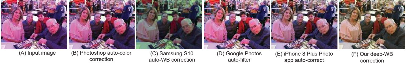
Figure 9: Strong color casts due to WB errors are hard to correct. (A) Input image rendered with an incorrect WB setting. (B) Result of Photoshop auto-color correction. (C) Result of Samsung S10 auto-WB correction. (D) Result of Google Photos auto-filter. (E) Result of iPhone 8 Plus built-in Photo app auto-correction. (F) Our AWB result using the proposed deep-WB editing framework. Photo credit: OakleyOriginals Flickr-CC BY 2.0.
