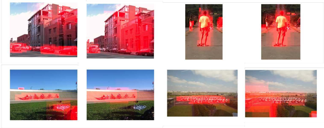
Figure 6. In each image we show the distribution of the proposals produced by pasting a red box for each proposal. Only the top 100 proposals are shown. For each pair of images, DeepBox is on the left and Edge boxes is the right. DeepBox proposals are more tightly concentrated on the objects. See Section 4.3 for a detailed discussion.
