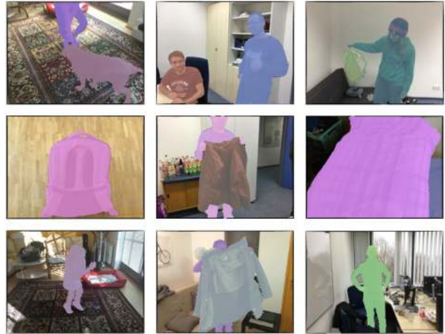
Figure 2: Our large-scale dataset contains a large variety of dynamic sequences with segmentation masks and point correspondences between different RGB-D frames.
