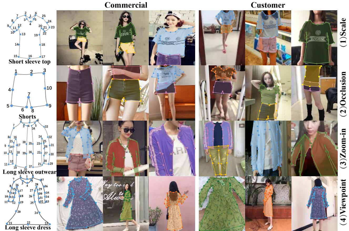
Figure 2. Examples of DeepFashion2. The first column shows definitions of dense landmarks and skeletons of four categories. From (1) to (4), each row represents clothes images with different variations including ‘scale’, ‘occlusion’, ‘zoom-in’, and ‘viewpoint’. At each row, we partition the images into two groups, the left three columns represent clothes from commercial stores, while the right three columns are from customers. In each group, the three images indicate three levels of difficulty with respect to the corresponding variation, including (1) ‘small’, ‘moderate’, ‘large’ scale, (2) ‘slight’, ‘medium’, ‘heavy’ occlusion, (3) ‘no’, ‘medium’, ‘large’ zoom-in, (4) ‘not on human’, ‘side’, ‘back’ viewpoint. Furthermore, at each row, the items in these two groups of images are from the same clothing identity but from two different domains, that is, commercial and customer. The items of the same identity may have different styles such as color and printing. Each item is annotated with landmarks and masks.
