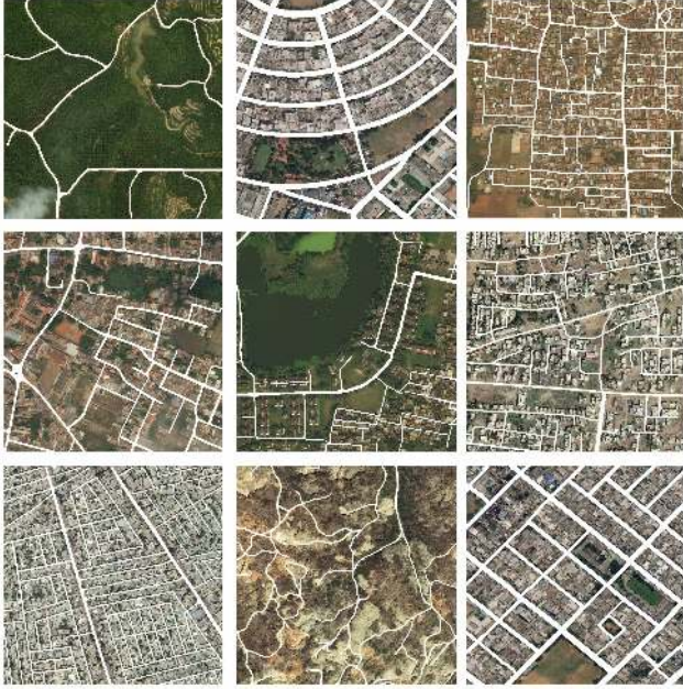
Figure 2: Road labels are annotated on top of the satellite image patches, all taken from DeepGlobe Road Extraction Challenge dataset.
