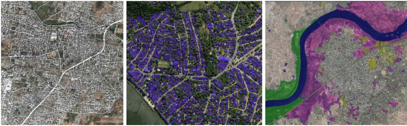
Figure 1: DeepGlobe Challenges: Example road extraction, building detection, and land cover classification training images superimposed on corresponding satellite images.
