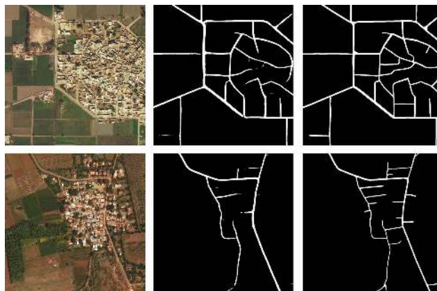
Figure 4: Example results of our road extraction method with an IoU score of 0.545, with satellite image (left), extracted road mask (middle), and the ground truth (right).
