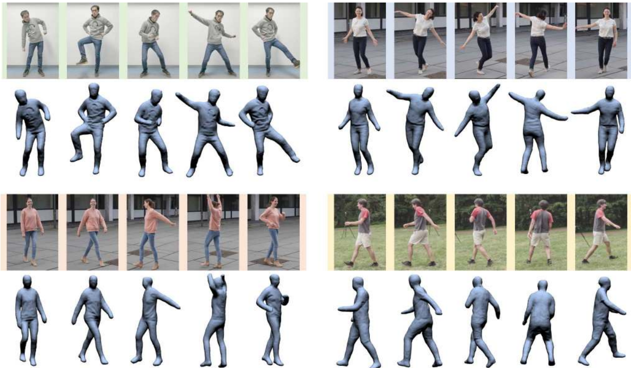
Figure 6: 3D reconstruction from monocular videos using our method. The reconstruction results are generated by applying our method on each individual video frame independently. The last three video clips come from the dataset of MonoPerfCap[59].
