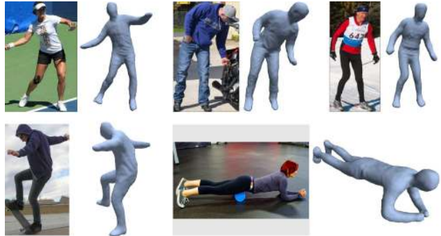
Figure 1: Given only a single RGB image, our method automatically reconstructs the surface geometry of clothed human body.
