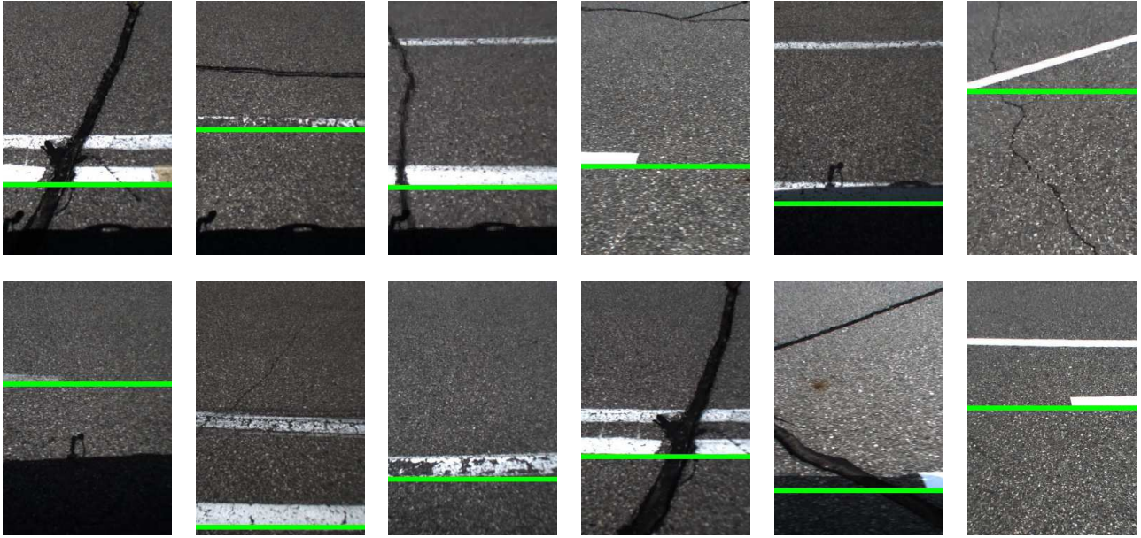
Figure 12: This figure shows lane marker positions estimated by the DeepLanes network. The network is able to detect lane markers that are in the shadow as well as parallel, broken and scattered markers.
