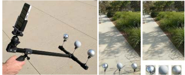
Figure 3: Left: Capture apparatus. Center: Example frame. Right: Processed data (top: input; bottom: ground truth).
