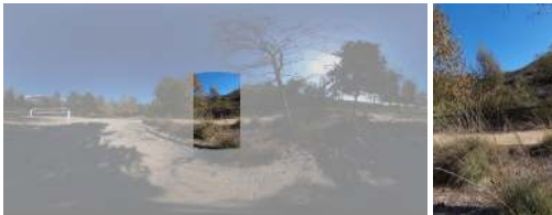
Figure 2: The field of view (FOV) of mobile phone video (inset shown in full color), relative to the 360° environment.
