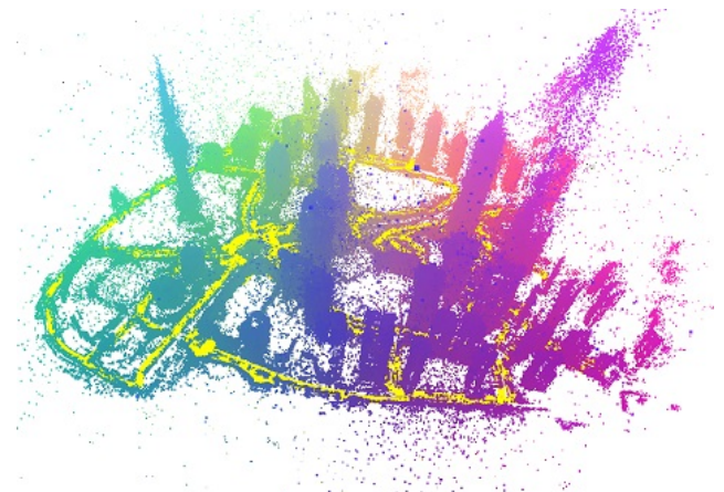
Figure 1. Large-scale bundle adjustment on a deep learning framework using stochastic domain decomposition. We solve problems on a very large scale with high convergence quality.
