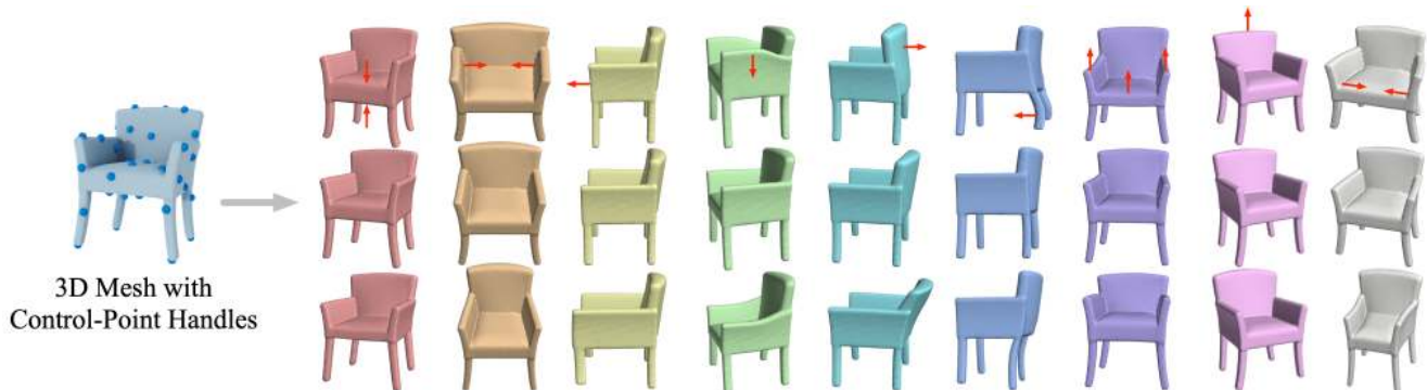
Figure 1: Learned meta-handles for a single chair. Each column indicates a meta-handle and shows three deformations along the direction of that meta-handle, with red arrows highlighting the deformed region. Our method learns intuitive and disentangled meta-handles in an unsupervised fashion, which factorize all the plausible deformations for the shape.
