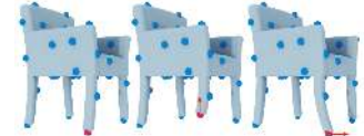
Figure 2: Two deformations resulted from moving the red control point along the arrow directions.
