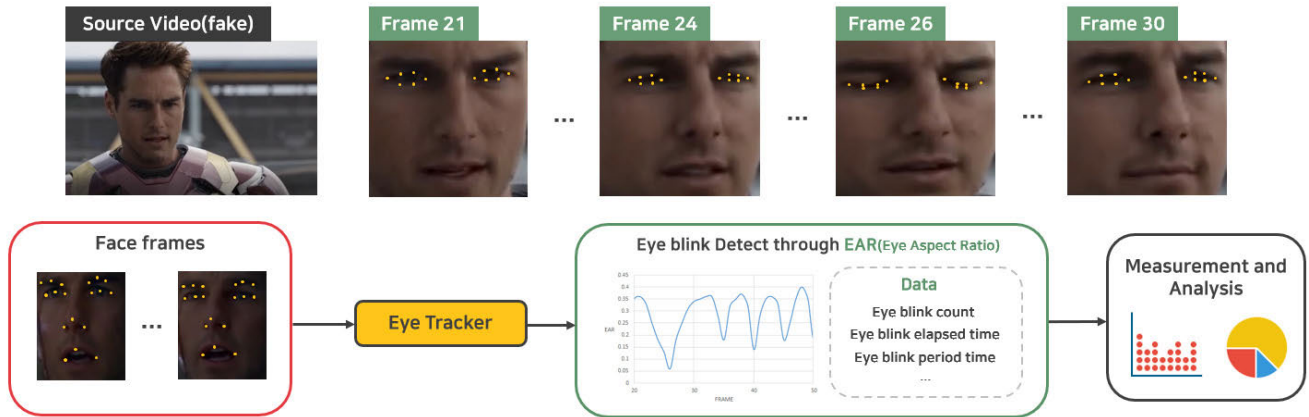
FIGURE 5. This is a visualization of DeepVision’s eye tracker. It is able to measurement the blinking count, period, and more through the EAR (Eye-Aspect-Ratio) algorithm.
